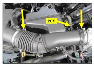
2. Loosen the clamps on the intake tube and disconnect the PCV breather. Remove the intake tube and set it aside.
